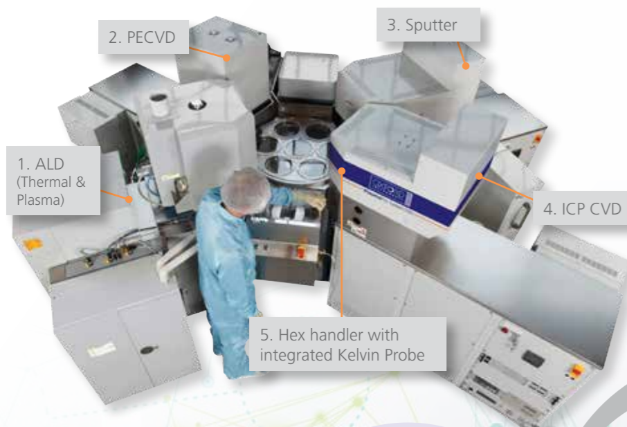
OpAL system in glovebox for handling moisture sensitive samples
