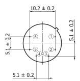
Distance from photosensitive area center to cap center -0.3≤X≤+0.3 -0.3≤Y≤+0.3
