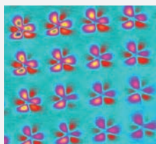
FeCr Ferromagnetic Nanostructures, 6.5 \times 6.5\mu\text{m}
