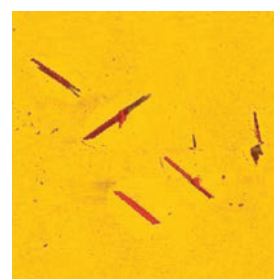
Needle-like crystals of azobenzene derivative formed from monomolecular LB-layer on silicon surface at 75^{\circ}\text{C} . Scan size: 32 \times 32\mu\text{m}
