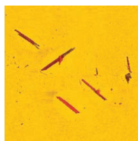
Needle-like crystals of azobenzene derivative formed from monomolecular LB-layer on silicon surface at 75^{\circ}\text{C} . Scan size: 32 \times 32\mu\text{m}
