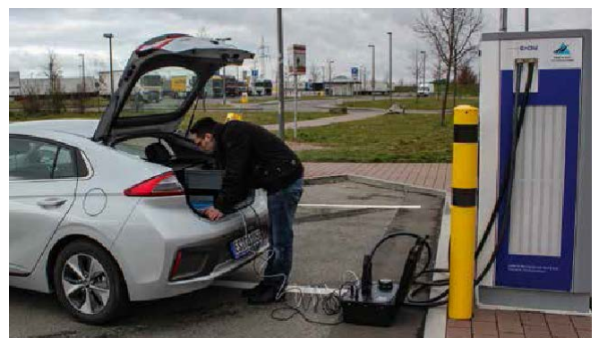
Compact, robust design for comfortable outdoor use. In this picture you can see a DC-CCS test.
