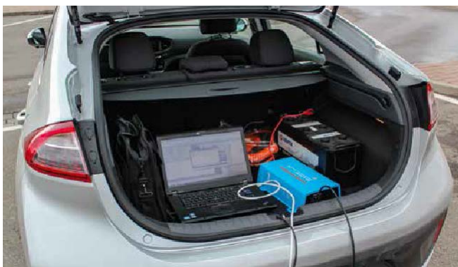
Laboratory in your case: Laptop, inverter (12V to 230V) and battery. (Components not supplied by comemso.)
