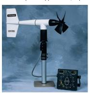
Wind Sensor Interface offers calibrated 0-5VDC outputs for wind speed and wind direction. Model 05631C Wind Line Driver provides calibrated 4-20 mA current signals for each channel, useful in high noise areas or for long cables of up to several kilometers. Each interface circuit is supplied in a weatherproof junction box with mounting hardware for installation near the sensor.
