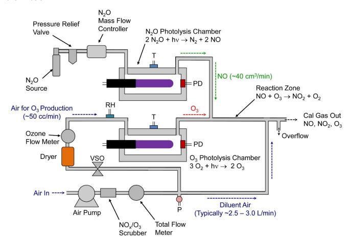
For the production of ozone, a small flow of scrubbed and dried ambient air is directed into the  $O_3$  photolysis chamber (lower part of the diagram). The vacuum UV emission lines of a low-pressure mercury lamp near 185 nm are absorbed by  $O_2$  to produce oxygen atoms, and the oxygen atoms rapidly attach to  $O_2$  via a collisionally stabilized reaction to form  $O_3$ . The well-known mechanism, which also is responsible for the presence of Earth's protective ozone layer, is as follows:
