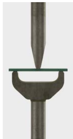
3-point bending 40 mm
