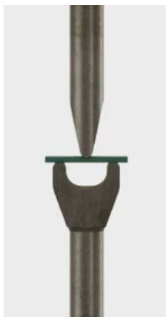
3-point bending 20 mm
