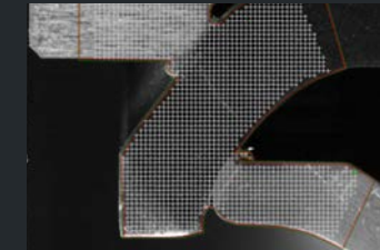
非镶嵌样表面测试点阵 Test point pattern on a non-bedded specimen
