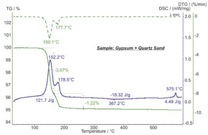
The measurement was carried out at a heating rate of 10 K/min under an air atmosphere in the SiC furnace. The sample mass amounted to 34.30 mg.
