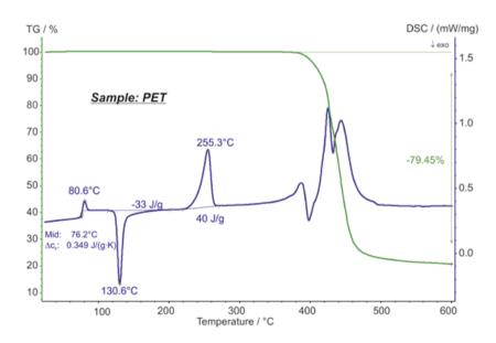
The SiC furnace was used for the investigation of the thermal behavior of a PET sample (10.13 mg) in a nitrogen atmosphere. The heating rate amounted to 10 K/min.
