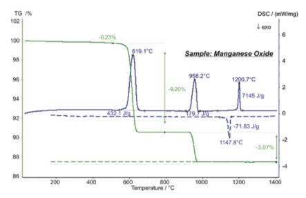
This STA measurement was carried out in the rhodium furnace under an air atmosphere. The oxide (32.14 mg) was heated at a rate of 20 K/min.
