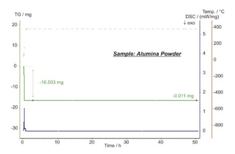
The long-term measurement on an alumina powder was performed at 400°C over 50 hours in the platinum furnace.
