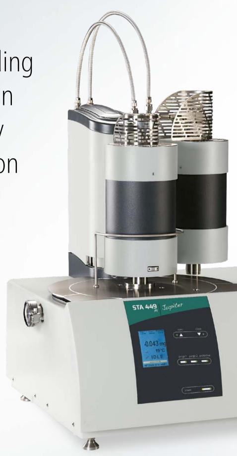
The STA 449 **F1** Jupiter® combines a high-performance Heat-Flux DSC with a nanogram-resolution thermobalance, thereby offering a high sample load and wide measurement range. This STA system can easily be adjusted to nearly any possible application by selecting the optimum furnace, installing the most appropriate sensor and using the proper accessories. It is a unique and ideal tool for material characterization in research and development.
