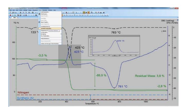
User interface during evaluation: TGA curve (green line) together with the DTG curve (black dotted line), DSC curve (blue line), two curves representing the gas flow of nitrogen (red dotted line) and synthetic air (blue dotted line); PIP presentation (picture-in-picture) for the DSC peak at 423°C.
