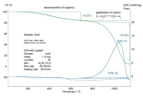
For these tests, the water-vapor furnace was used for one measurement in a nitrogen atmosphere (dashed lines) and a second measurement in water vapor (100%; solid line). The sample masses amounted to approximately 6 mg; heating rates to  $20 \, \text{K/min}$ .
