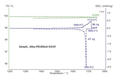
This dental alloy (202.13 mg) was measured in the graphite furnace in an argon atmosphere and at a heating rate of 10 K/min.
