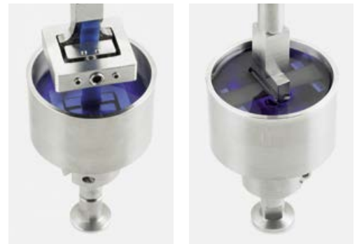
Sample holder for tensile tests (left) and bending tests (right) in an immersion bath
