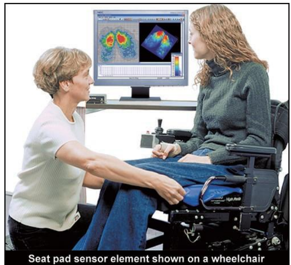
Seat pad sensor element shown on a wheelchair
