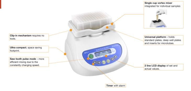
Supplied with a platform to allow vortexing of single tubes and skirted plates. Additional inserts for microtubes sold separately or available as part of MPS-1-K (see page 9.8).
