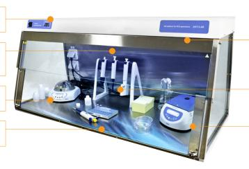
Built-in UV cleaner recirculator increases the maximum density of UV light and generates 25 m³/h air flow exchange – prevents unwanted contamination and protects the user from direct UV light (in the upper hood) during manipulation.
