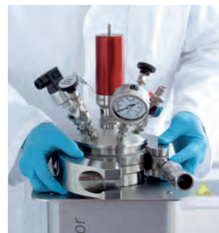
Easy-to-use clamping rings and chains for secure closure
