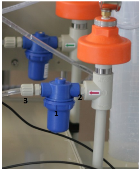
Fig. 16: Application example on a bench scale pump unit: The filter (1) is mounted with the screw connection (2) at the T-piece of the pressure measurement device. The hose connection (3) is screwed into the filter body and connects the hose in direction to the ED stack.
