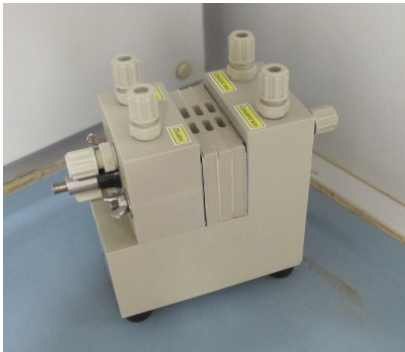
Fig. 18: A micro ED with three open center chambers for measurement of voltage drop and membrane potentials.
