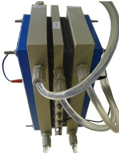
Fig. 14: ED 200 with center electrode and two stages on the right side of center electrode and one stage on the left side of electrode. Flow from right to left.
