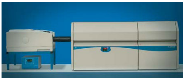
PL-GPC220 与 Perkin Elmer Spectrum One FTIR 连接
