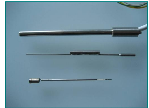
Push Rod with body (above), purge gas line (middle) heater assembly (below)
