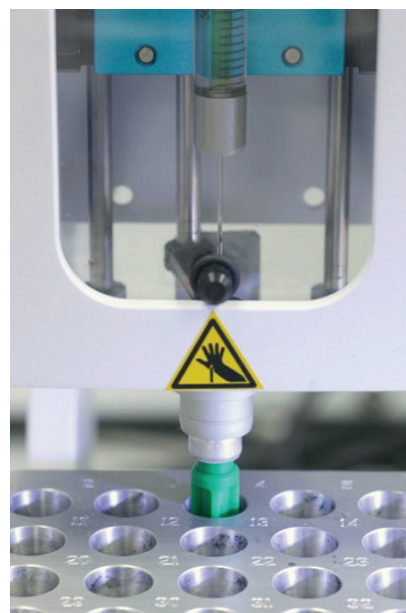
Figure 3: Elution of QuEChERS extract through an ITSP cartridge, using the aluminum tray cover.
