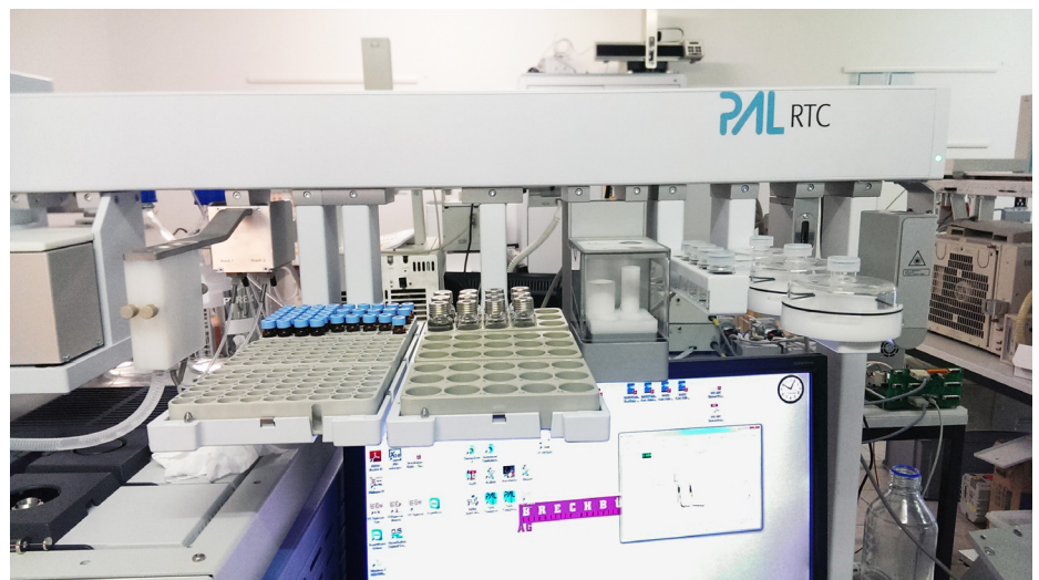
Figure 1b: The PAL RTC with (from left to right) incubator, fast wash station, VT54 trays, VT15 trays, vortex mixer, standard wash, solvent station, bar code reader.
