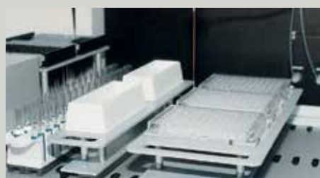
Tecan Freedom EVO®-based locating pins provide compatibility with most Freedom EVO strip racks, reagent troughs and microplate racks.
