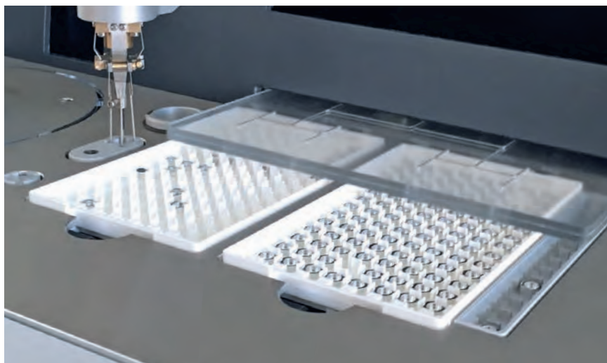
Two interchangeable pan trays plus one fixed strip yield a total of 204 positions for sample and reference pans; these are displayed here with the tray cover partially opened. Each tray can carry sample and reference pans of different types.
