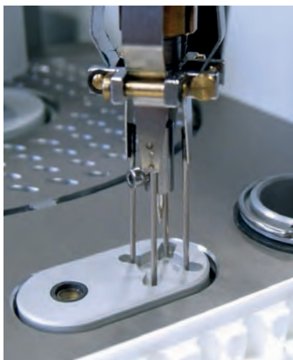
Gripper with piercing device and photo diode (left) for pan recognition "on the fly"
