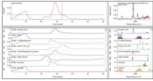
The top left panel shows the Gram-Schmidt reconstruction indicating a material is being evolved during the thermal decomposition of the resin. The lower right panel is from the result of the Mercury TGA analysis algorithm automatically identifying the compounds present in the Gram-Schmidt reconstruction. The lower left panel displays the profiles showing which materials are being evolved at a given time.
