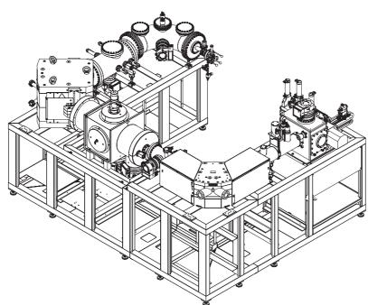
Ionplus is currently developing a low-energy Multi-Isotope AMS instrument in collaboration with ETH Zurich. The new instrument will cover <sup>10</sup>Be, <sup>14</sup>C, <sup>26</sup>Al, <sup>41</sup>Ca, <sup>129</sup>I, U and Pu and combines accelerator and ion source technology of the MICADAS system with the concept of the high-energy spectrometer layout of the 600 kV "TANDY" facility at ETH.
