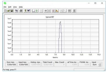
measurement curves. Important measurement data, including count rate, count maximum, position and peak width are continuously displayed. A comprehensive online help system eases the user into fully employing the capabilities of the MultiHarp 150. A library for custom programming, e.g., with LabVIEW is also included. PicoQuant is committed to the support and development of this software and upgrades with extended functionality will be made available.
