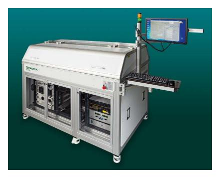
Main laser feature is output of temporary shaped pulses based on electrooptical modulator driven by programable arbitrary wave generator (AWG). Pulse shaping resolution is 125 ps and pulse duration up to 50 ns. Start of the system is a single mode CW laser. Then light is amplified in fiber amplifier, later AWG driven modulator transmits only required temporal shape and duration pulse which is amplified in diode pumped regenerative amplifier in order to reach energy level sufficient to amplify
