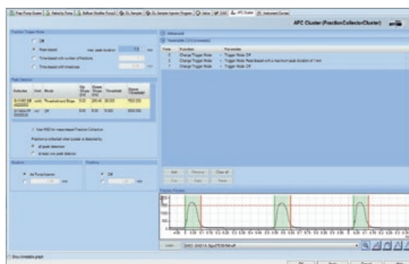
Multiple collection modes are possible and the fraction preview in Agilent OpenLAB CDS makes it easy to determine the correct trigger parameters.
