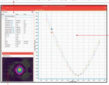
This window displays the 2D or 3D beam profile of the currently measured point in the beam propagation curve. This image enables visual intuitive verification of the beam profile behavior through focus. After each run the user can click any individual measured point and observe the beam profile. Outlying or anomalous points can be automatically or manually excluded from the curve fit calculations for more accurate results
