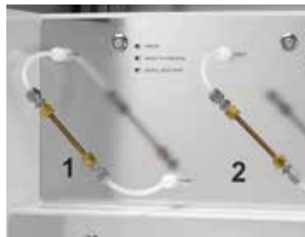
VOC trapped by Tenax tubes
