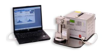
The instrument includes pumps, butanol tank, battery, internal memory, and the option for remote operation. The model 5403 provides highly accurate measurements for nanoparticles as small as 4.5 nm over a wide concentration range of up to 10<sup>7</sup> particles/cm<sup>3</sup>.
