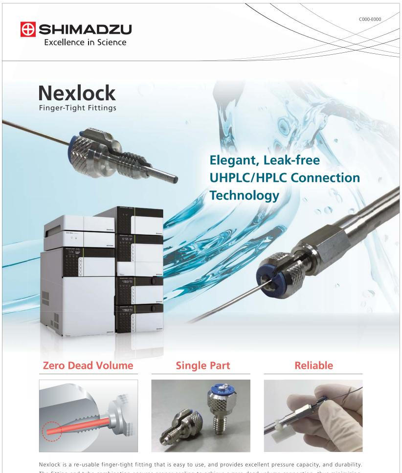
Nexlock is a re-usable finger-tight fitting that is easy to use, and provides excellent pressure capacity, and durability. The fitting and tube combination ensures proper sealing to achieve a zero dead volume connection, thus minimizing peak broadening and tailing. It withstands pressures up to 130 MPa without the use of tools.
