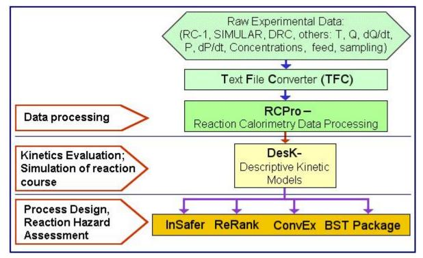
**RCPro** provides processing of data that include heat generation, pressure and concentration responses. Data can be generated by experiments run in BATCH or semi-BATCH mode with multi-component reacting mixtures. The auxiliary Text File Converter program allows simple method for data conversion. RCPro can be used in combination with any available reaction calorimeter.
