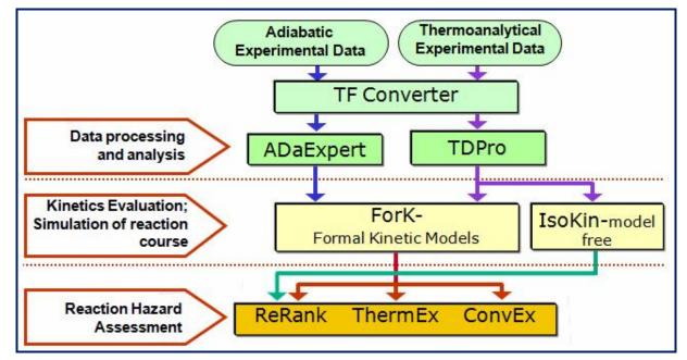
**TDPro** and **ADaExpert** support all necessary types of data processing for data of thermal analysis and adiabatic calorimetry. The auxiliary Text File Converter program allows simple method for data conversion so that TDPro and ADaExpert can be used in combination with any thermal analytical and adiabatic instrument respectively.
