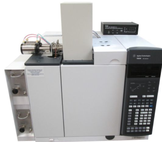
Figure 5 – Dual Liquid Petroleum Gas (LPG) Sampling Panels
