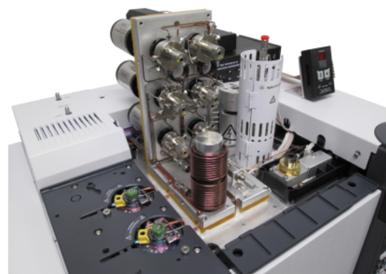
Figure 5 – Acid Gas and Trace Sulfur Auxillary Oven
