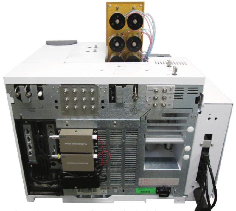
Figure 9 – Rear Mounting of Pulsed Discharge Modules with Custom Sampling Panels
