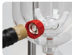
PTFE Stirrer Guide provides whip-free agitation
