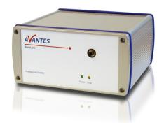
For high sensitivity applications where high resolution is not of paramount concern, the AvaSpec-HS2048XL-EVO is an exceptional instrument. Featuring Avantes' HS optical bench which has a full 0.22 numerical aperture for superior throughput, the AvaSpec-HS2048XL has a back-thinned CCD detector with 2048 pixels measuring 14X500 microns.
