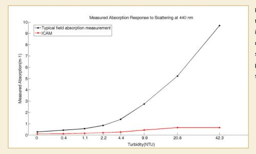
ICAM's patented design allows researchers to measure absorption with very little or no interference from particle scattering, maximizing measurement accuracy. Data show a minimal effect from scattering particles on ICAM's response versus typical spectrophotometric response.
