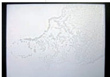
LABS-Test, which tests for silicone contamination, of a silicone containing sample
