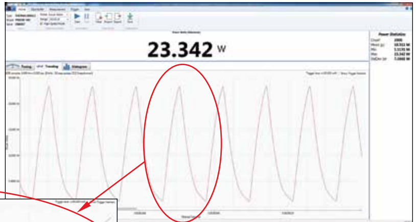
Pulse shape visualization obtained with a PowerMax-Pro sensor and LabMax-Pro electronics and software
