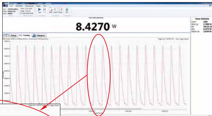
The new LabMax-Pro offers a "Snapshot Mode" which enables visualization of pulses as short as 10 \mu\text{s} and at high duty cycles
