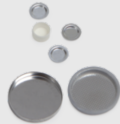
Coin cell case used as a large DSC crucible (with other typical DSC crucibles)
