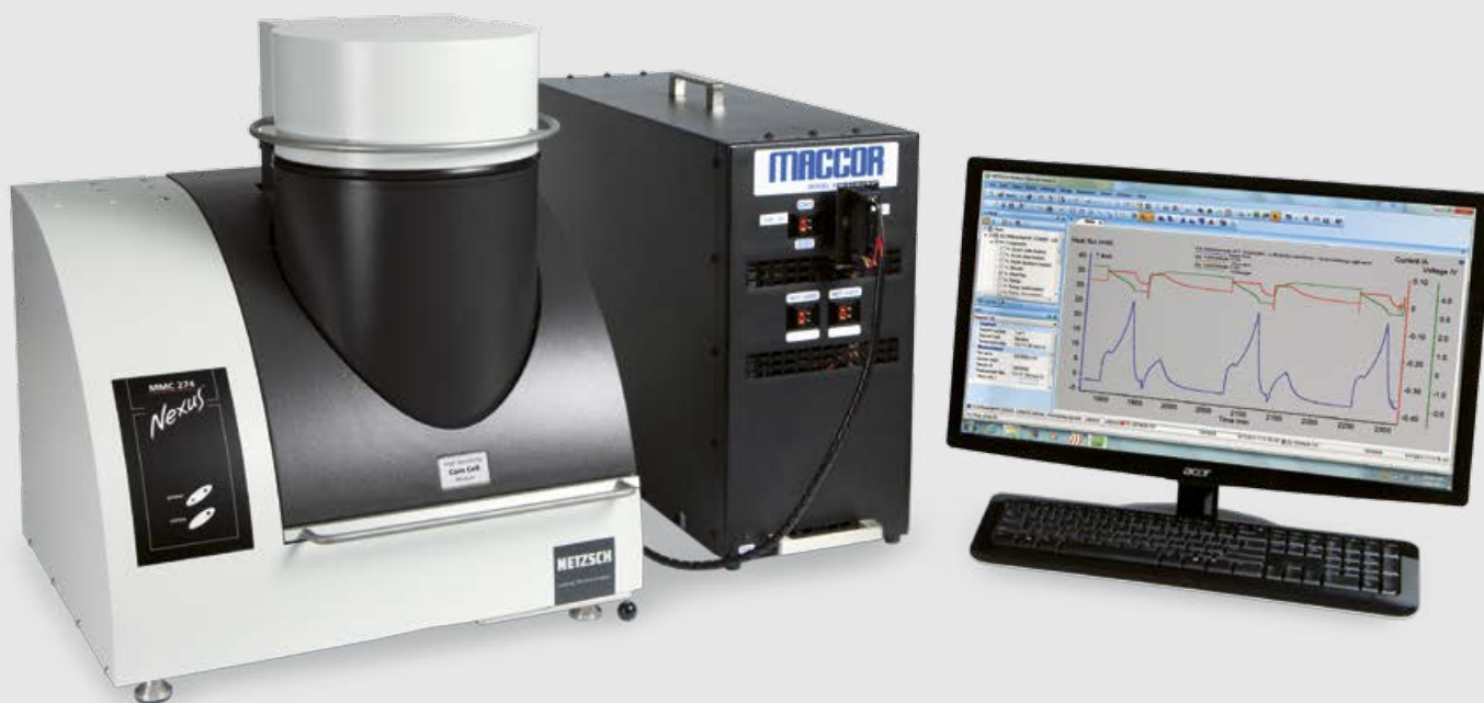
MMC with HT coin cell module with battery cycler
