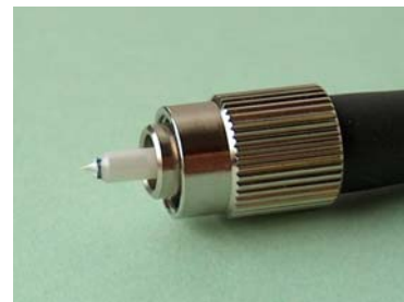
Figure 4.6.3: same connector as Figure 4.6.2 with heat conducting paste
