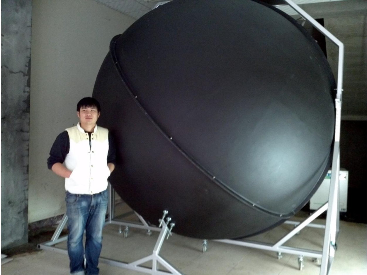
Fig 3. 3m diameter integrating sphere for Tokushima Centre of Measurement, Japan
