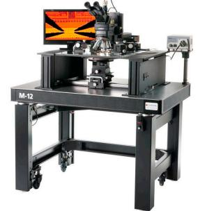
M12 manual probe system configured above with a Rapid Advance wafer chuck, 300 mm chuck, fixed platen, DC manipulators, compound optics, CCTV system, test instrumentation mounted on a vibration isolation table several configurations available.
