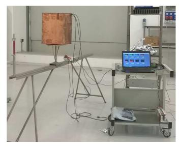
**SP2** is the ideal device for performing active neutron spectrum measurements in every radiation environment, including mixed stray radiation fields, workplaces characterized by high gamma background and reference calibration laboratories.
