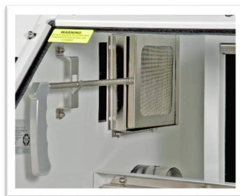
Figure 22: Catalyst Cartridge Installed
