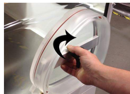
Figure 24: Securing the Arm Port Doors
