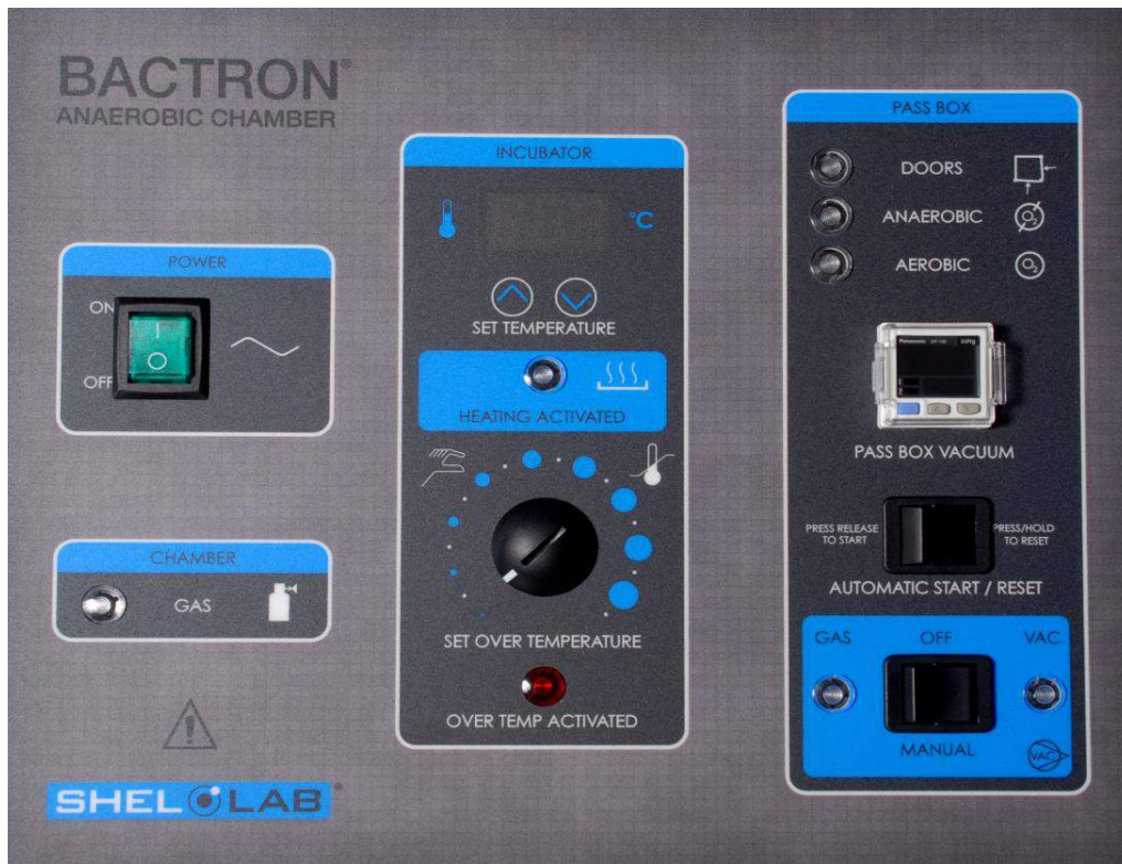
Figure3: Main Control Panel
