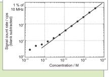
intensity decreases linearly with the concentration down to 50 pM. Below this concentration, the weak, parasitic fluorescence of the glass filter must be taken into account. Performing a blank measurement with the pure solvent as a sample and subtracting this blank measurement from the TCSPC histograms allowed a single exponential lifetime analysis at picomolar concentrations.
