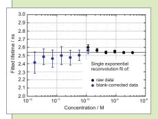
To demonstrate the sensitivity of the FluoTime 100, a set of very diluted solutions of Coumarin 6 in Ethanol was measured. The samples were excited at 10 MHz repetition rate with the LDH-P-C-405 diode laser. The average excitation intensity in the sample volume was 80  $\mu$ W. Magic angle polarized fluorescence was collected through a 530 nm longpass filter. The detected
