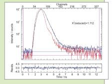
PMA 182 detector. The FluoTime 100 was equipped with sheet polarizers. The figures show the recorded polarized decays, the IRF of the measurement and the calculated fluorescence anisotropy decay. Fitting the anisotropy decay to a single exponential model without reconvolution yields 1.9 ns and 270 ps rotational correlation time of Coumarin 6 in EtGly and DMSO, respectively. The results reflect the different viscosity of the solvents.
