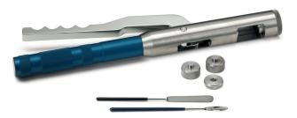
The PIKE Technologies Hand Press is an ideal solution for laboratories that require only occasional preparation of KBr pellets and cannot justify the expense of a hydraulic press.
