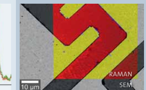
Raman-SEM image overlay of a LT GaAs sample. In the color-coded Raman image the gold substrate (yellow) can be clearly distinguished from GaAs (red) correlated with the ultra-structure of the sample. Raman image: 50 x 50 μm², 300 x 300 pixels = 90,000 spectra, 34 ms integration time per spectrum. (1)
