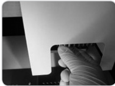
3. Put Silicon Grease on O-rings (black rubber rings) on Nozzles.
